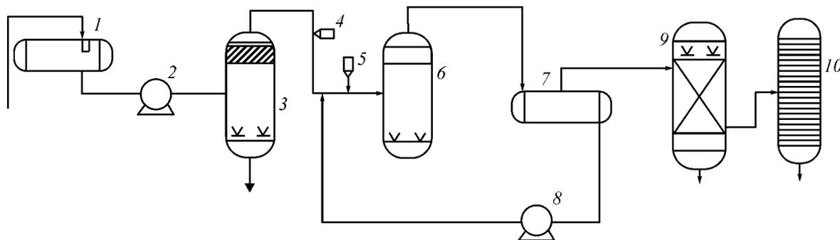
Scheme of an installation for catalytic oxidation of sulfur-containing compounds of the pentane–isopentane fractions with atmospheric oxygen: (1) receiver for raw material, (2, 8) pump, (3) column for preliminary alkali washing, (4) compressed air, (5) vessel with catalyst, (6) mixer, (7) settler for alkali, (9) sand filter, and (10) distillation column.
